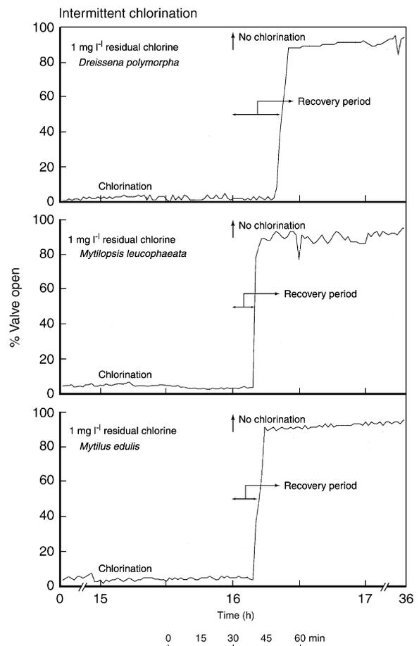
Fig. 4. Mussel-monitor<sup>®</sup> data (magnified between 15 and 17 h in Fig. 3) showing recovery period (between cessation of chlorination and resumption of feeding) in *Dreissena polymorpha*, *Mytilopsis leucophaeata* and *Mytilus edulis* during intermittent chlorination. ↑ denotes stoppage of chlorine.
