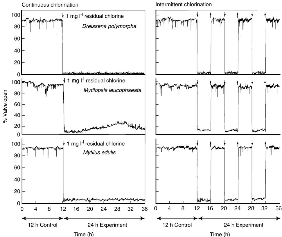
Fig. 3. Average ( $n = 6-7$ ) patterns of shell valve movements of *Dreissena polymorpha*, *Mytilopsis leucophaeata* and *Mytilus edulis* subjected to continuous and intermittent chlorination (4 h on and 4 h off cycle) at  $1 \text{ mg l}^{-1}$  chlorine concentration. The status of the shell valves was logged every 1 min. ↓ denotes addition of chlorine and ↑ denotes stoppage of chlorine.
